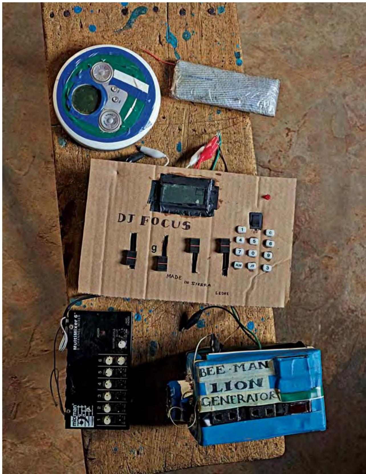
Kelvin Doe's homemade broadcast equipment, assembled from a salvaged CD player, improvised battery, mixer, and homemade generator. Freetown, Sierra Leone.
