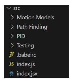
Inside the Motion Models folder, we have separated files into python\_versions and js\_versions which are the names of the two folders. Initially, when we receive a pseudocode, we translate it into Python. Then, after testing to make sure the code works in Python, we immediately translate the same code into JavaScript and this JavaScript code is the thing we import into the app.
